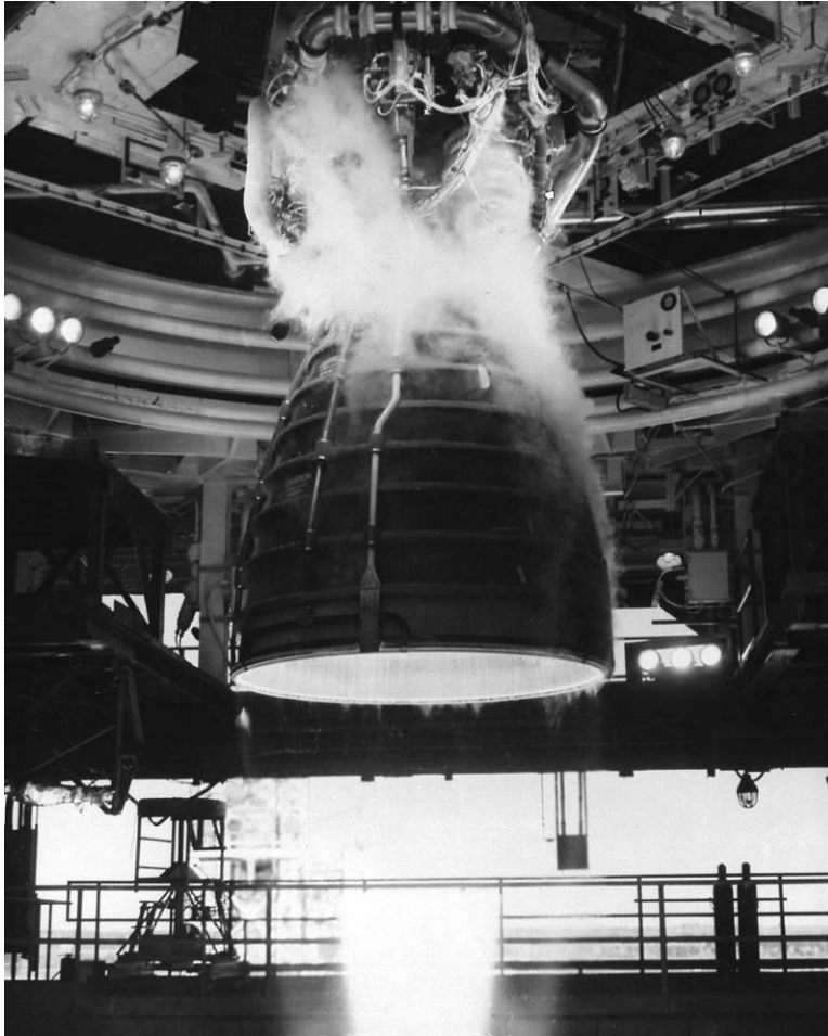
Figure C-13. Close-up view of a SSME test, direction unknown, April 1, 1979. Source: George C. Marshall Space Flight Center, Marshall Image Exchange (MIX), 7995081, accessed at http://mix.msfc.nasa.gov/ .
